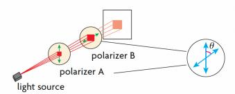
The amount of the reduction in light intensity, I, depends on  $\theta$ , the acute angle formed between the axis of polarizer A and the axis of polarizer B. Malus's law states that  $I = I_0 \cos^2 \theta$ , where  $I_0$  is the intensity of the initial beam of light and I is the intensity of the light emerging from the polarizing material.
