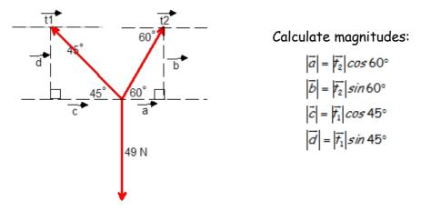
For the system to be in equilibrium, the magnitudes of the horizontal components must balance each other and the magnitudes of the vertical components must balance each other.
