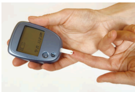
Figure 3 A glucometer gives a quantitative measure of the blood glucose level. A drop of blood is required for the analysis.
