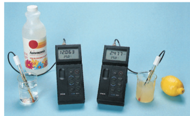
Figure 10 A pH meter shows the pH of a solution.
