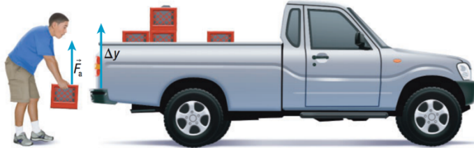
Figure 2 A worker applies a force F_a to a crate, doing work as he lifts the crate from the ground up to the truck bed. The change in height of the crate is \Delta y .
