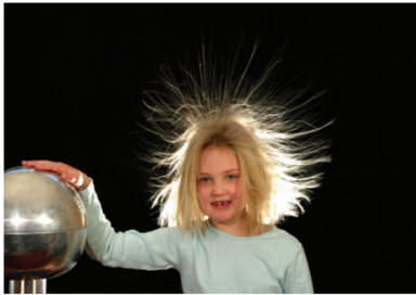
Figure 1 Electric charges on each strand of hair exert a repulsive force on the other strands, causing the hair to rise and spread out.
