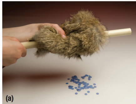
Figure 2 When a plastic rod is rubbed with fur (a), the rod acquires an electric charge. (b) The charged rod attracts small bits of paper and other objects.
