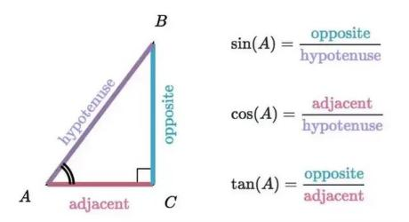
Based on the definitions of the three primary trigonometric identities as stated in the above diagram, by using the first character of each identity you will get SOH CAH TOA.
