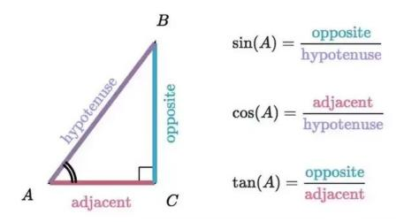
Find the values for sin(A), cos(A), tan(A) for a triangle with the lengths of these sides.
