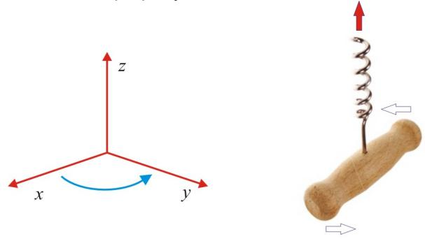
If you rotate the x-axis towards the y-axis using the shortest path, the screw goes in the positive direction of the z-axis.
